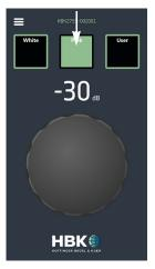
To change the attenuation, turn the attenuation knob by swiping the cursor from the bottom left to the top right and back again (click+drag on a laptop). While the changed attenuation value is being sent to the amplifier, the displayed value shortly turns red.
