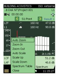
In the area below the spectrum, two parameters can be shown – both can be selected from drop-down menus, see Fig. 4.7.
