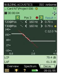
The Decay Parameter Selectors above the graph select which decay to display: T20@Pos or T30@Pos. Each of these selections show the decay for the measurement at the selected position together with the readout of T20@Pos and T30@Pos resp. T20 and T30 show the decay for the current position. If you only want one graph you can set the other selector to Off.
