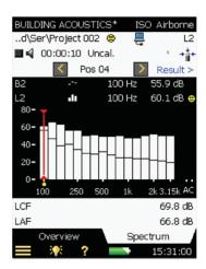
To select the frequency bands to be measured (using noise limited to cover these bands only), tap Main Menu > Setup > Measurement Control L1, L2 and B2 > Level Measurement Mode and select Serial.
