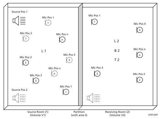
**L1** refers to the sound level measurements made in Source Room (1) – these are used in airborne and façade sound insulation calculations.
