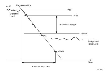
Reverberation time used in building acoustics is labelled either T20 or T30, depending on which of the two evaluation ranges were used.
