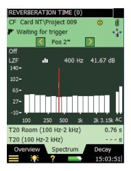
The main spectrum graph on the display (the bar graph) is selected using the parameter selector on the second line of the two shown above the graph (LZF in Fig. 4.26). The parameter selector for the main spectrum is linked to the selector on the **Overview** tab and the parameter selector for the main decay on the **Decay** tab.
